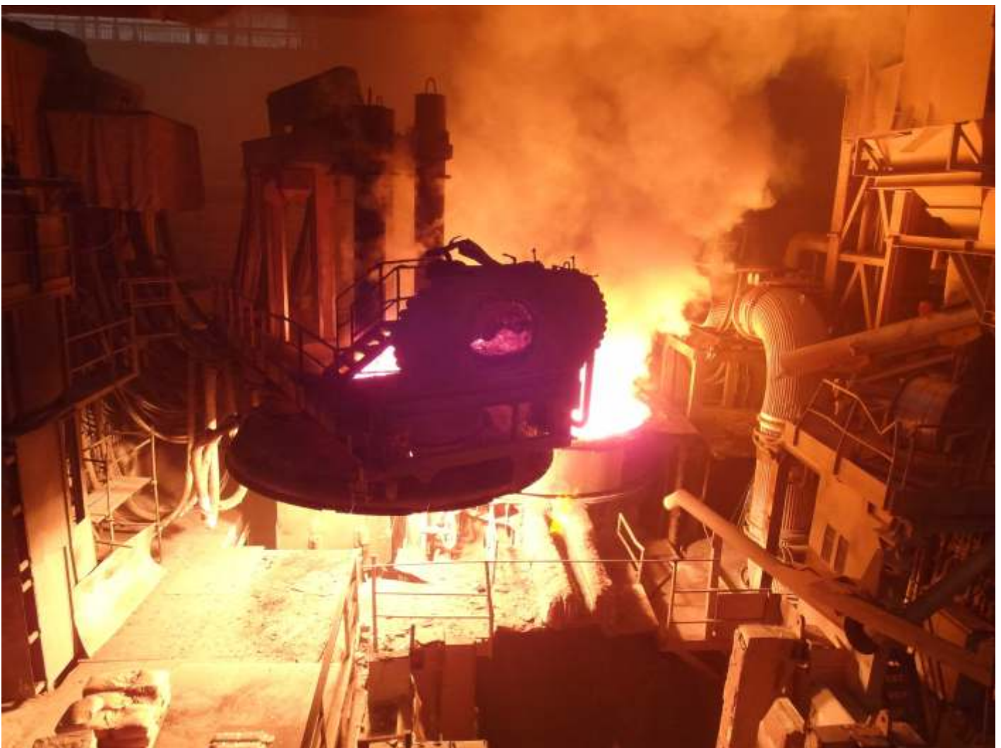
photo above: charging the electric arc furnace
