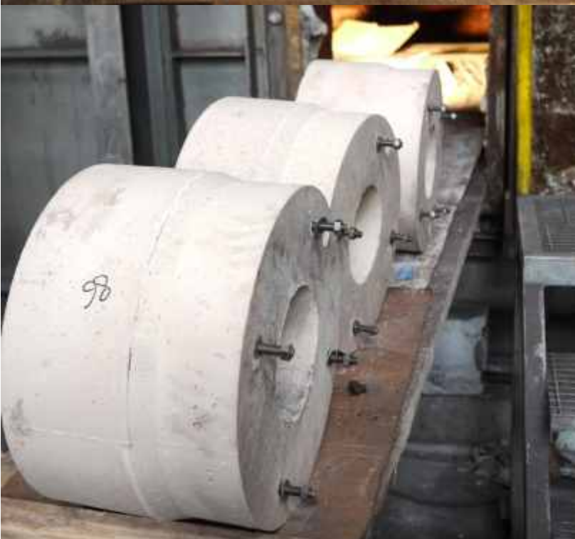
Above: the ceiling blocks are hang on a metallic construction; below: burners
