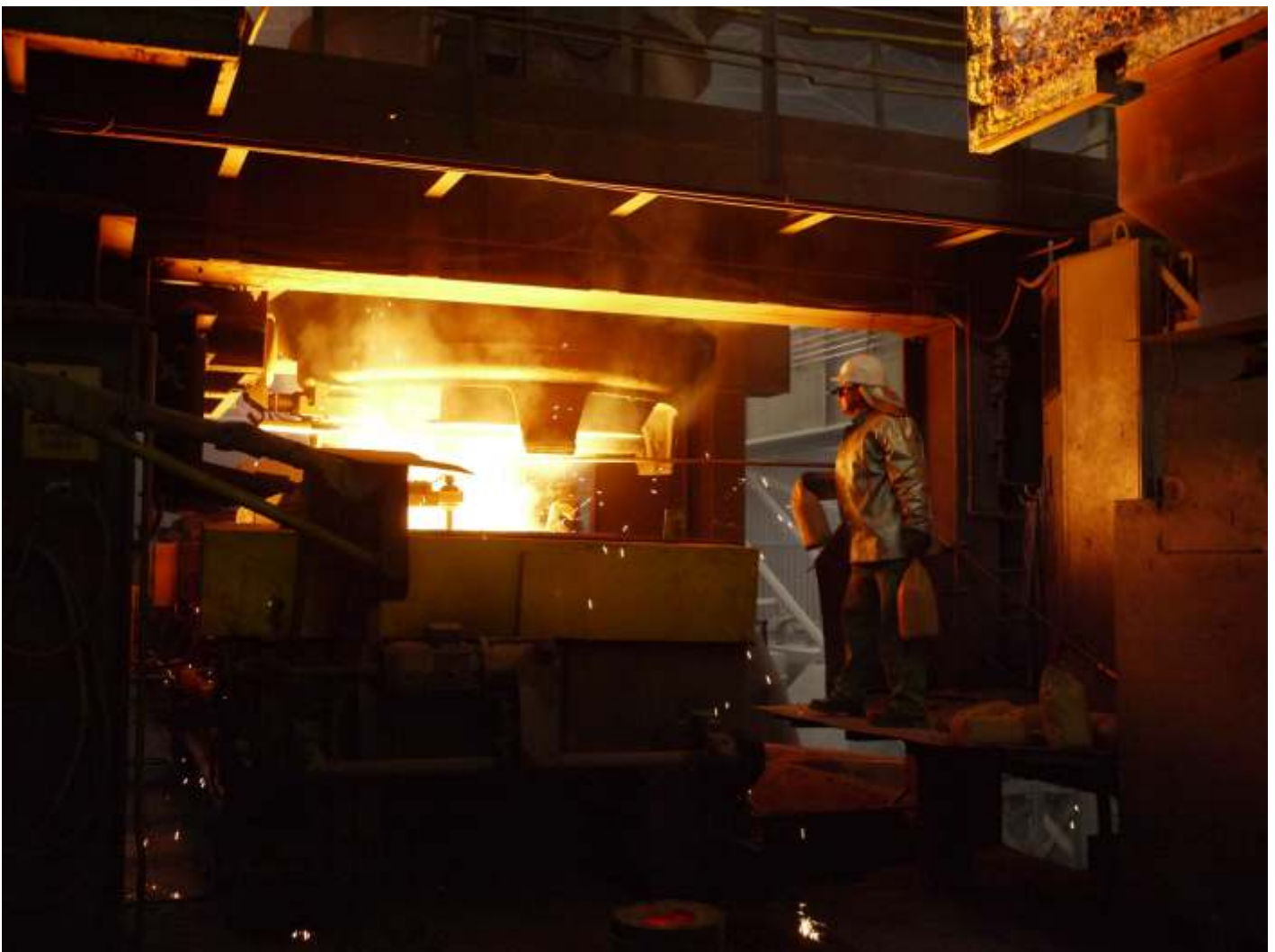
Photo: Pouring of steel from the ladle into the tundish on the existing continuous caster.
