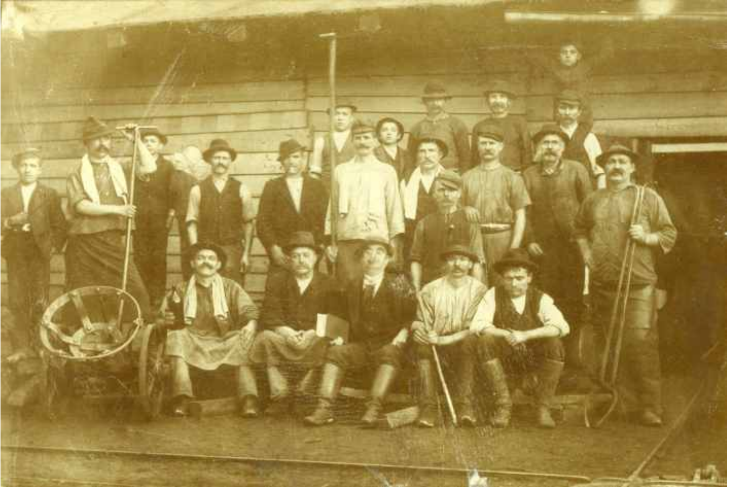
Group of puddlers with their tools and with trolley for transport of white-hot bloom from puddling furnace to hammers where it was prepared for further rolling; 1905, photography, from Železarski muzej Štore
